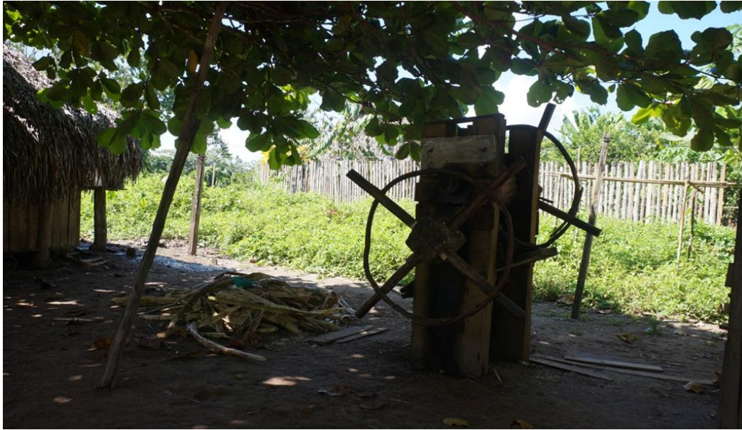
Figure 21 Mill used to squeeze out the juice from the stems of Saccharum officinarum ( Caña de azúcar )
