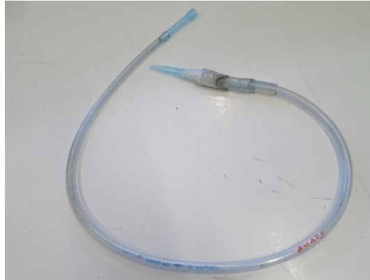
Figure 16: An aspirator used in the handling of O. thripoborus (Van De Walle, 2014)
