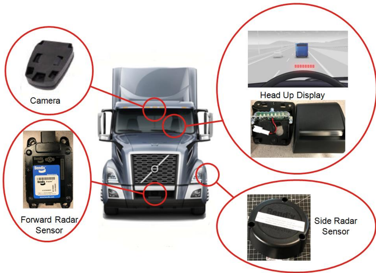
Figure 22: Key FCW/AEB components for the Volvo VNL (Bendix® Wingman® Fusion™ System)
