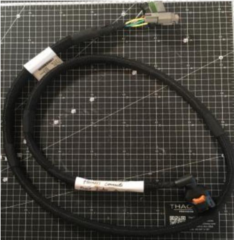
Bendix® Wingman® Fusion™ Head Up Display Side Sensor Radar Wire Harness (photo credit MeC S.r.l)
