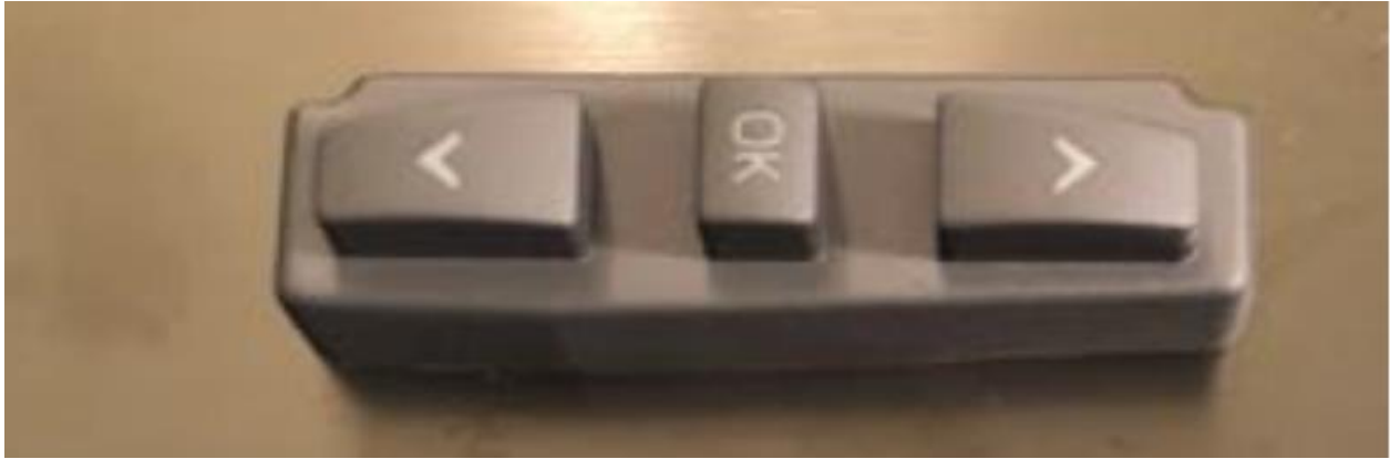
Bendix® Wingman® Fusion™ Driver Interface Unit (Display), Selection Buttons (photo credit: MeC S.r.l.)
