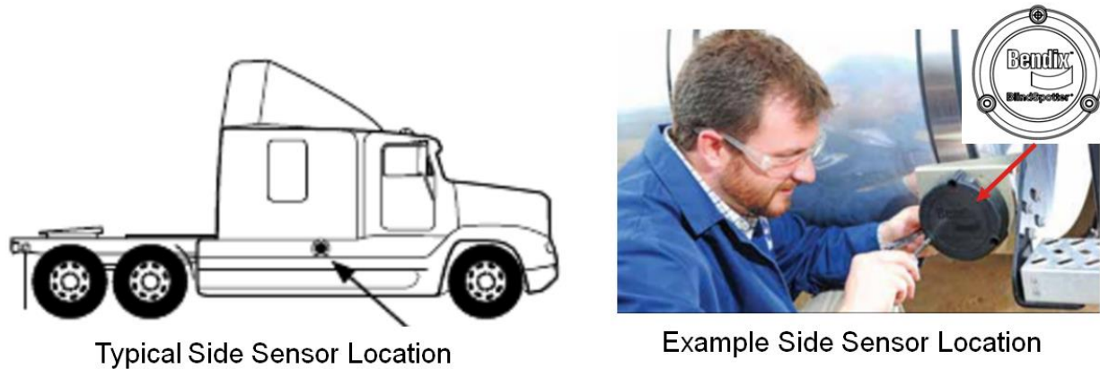
Figure 27: Typical Location of Bendix® Wingman® Fusion™ Side Radar Sensor (photo credit: Bendix Operator’s Manual)
