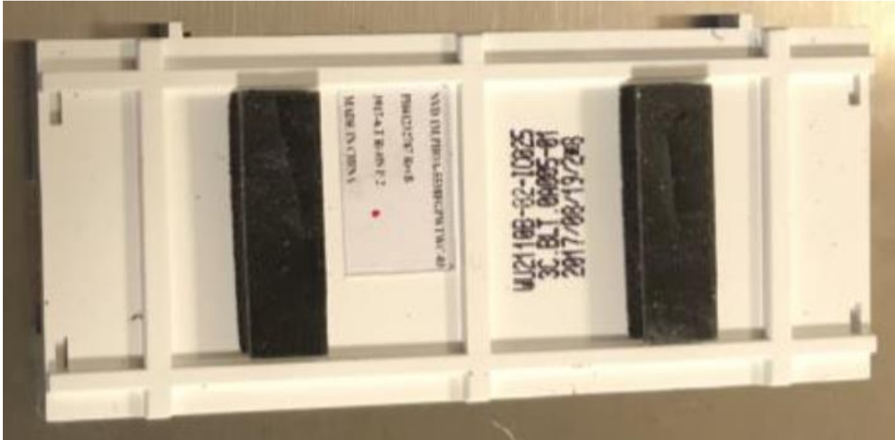
Bendix® Wingman® Fusion™ Driver Interface Unit (Display), LCD Display Assembly (photo credit: MeC S.r.l.)
