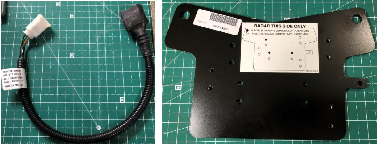
Meritor WABCO OnGuardACTIVE® Display Adapter Harness (left) and Radar Sensor Bracket (right) (photo credit MeC S.r.l)
