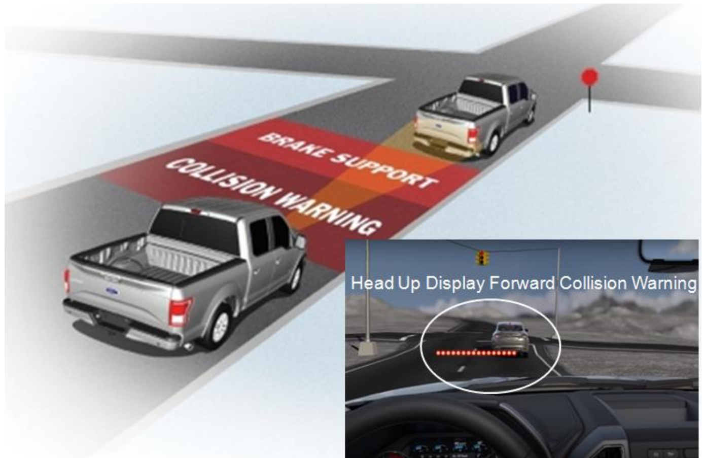
Figure 11: Ford FCW Zone, Brake Support Zone and Head Up Display (Reference: Ford 350 Super Duty® Owner's Manual)
