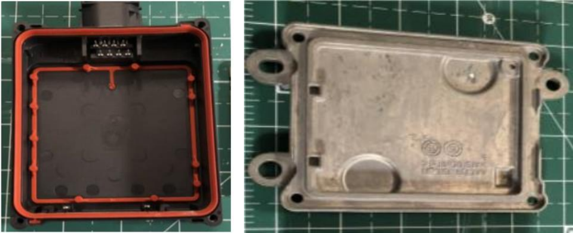
Freightliner Cascadia® Radar Housing Top (left) and Bottom (right) (photo credit MeC S.r.l)
