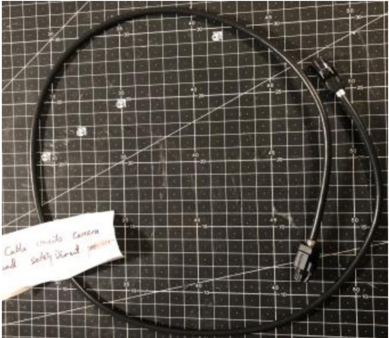
Bendix® Wingman® Fusion™ Cable and Connectors (connects to camera, SafetyDirect® Processor, and roof harness) (photo credit: MeC S.r.l.)
