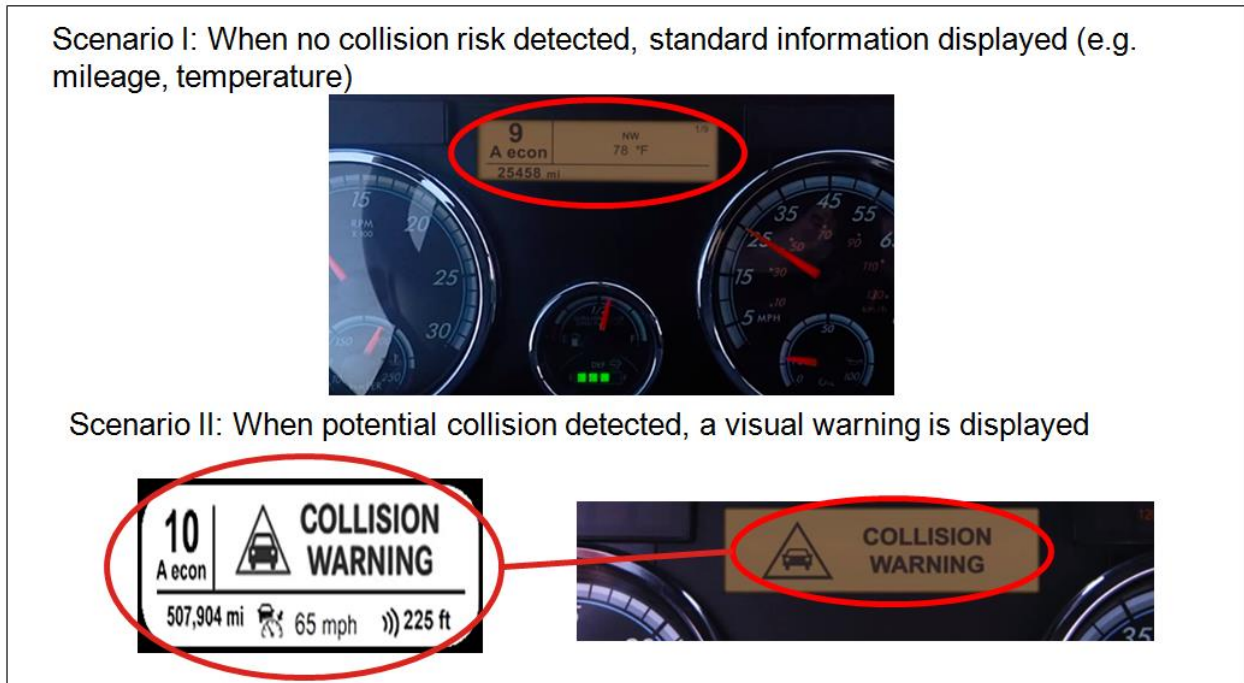
Figure 18: The Detroit Assurance® System utilizes the existing Cascadia® dashboard display (photo credit: Detroit Assurance® Brochure)
