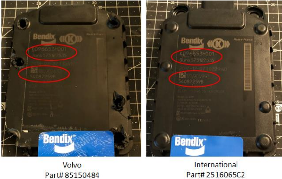
Figure 33: Comparison of Bendix® Wingman® Fusion™ Front Radar Sensor as employed by Volvo and International (photo credit: MeC S.r.l.)
