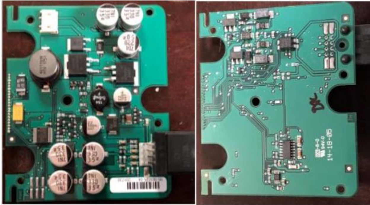
Bendix® Wingman® Fusion™ Driver Interface Unit (Display), PCB 1 Top (left) and Bottom (right) (photo credit: MeC S.r.l.)
