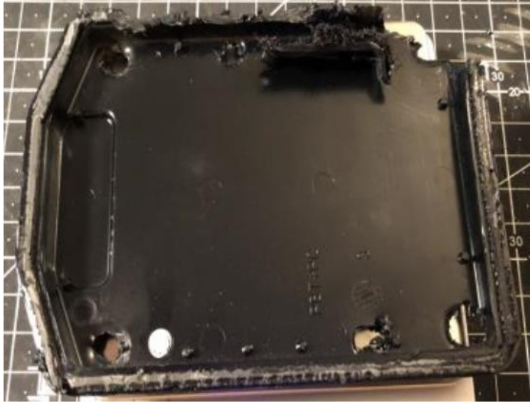
Bendix® Wingman® Fusion™ Head Up Display Front Sensor Bottom (photo credit MeC S.r.l)
