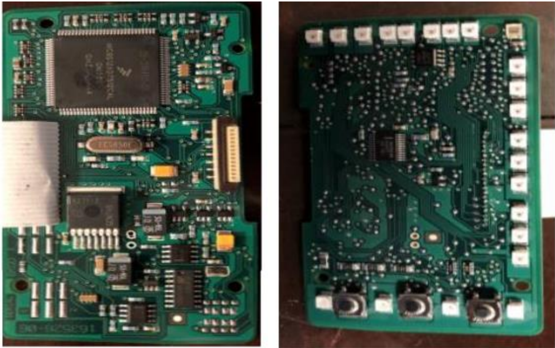
Bendix® Wingman® Fusion™ Driver Interface Unit (Display), PCB 2 Top (left) and Bottom (right) (photo credit: MeC S.r.l.)
