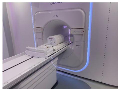
Fig. 1 ArcCheck MR on Elekta QA cradle on the Unity couch before a PSQA measurement
