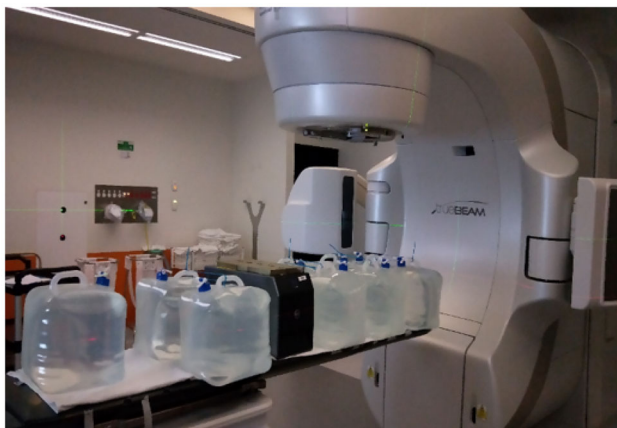
Figure 1: Load distributions, 158 kg to superior part and 70 kg to the inferior part of the couch
