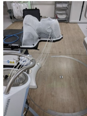
Fig. 17 Scalp treatment simulated using Steev phantom. Point dose measurement taken using PTW PinPoint chamber
