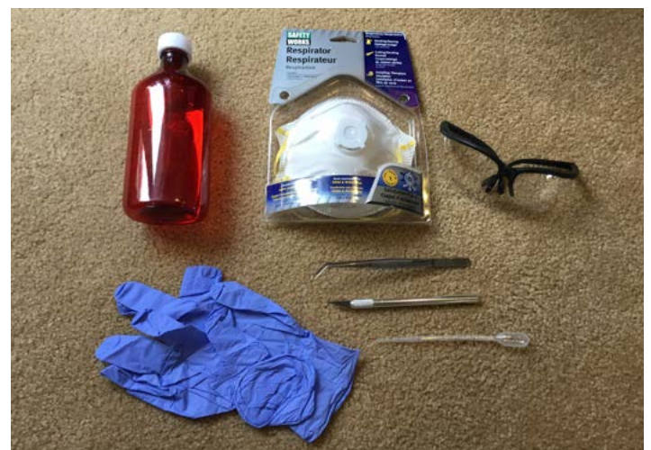
Above: Some materials and safety equipment... 400mL bottle, dust mask, safety glasses, nitrile gloves, forceps, X-Acto knife, and transfer pipette.
