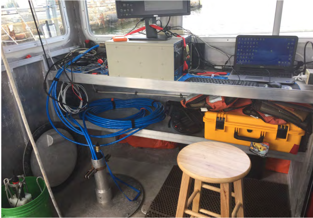
Figure 2.3-1 Geoswath setup on the RV Weicker, moonpool cover is in the lower left.
