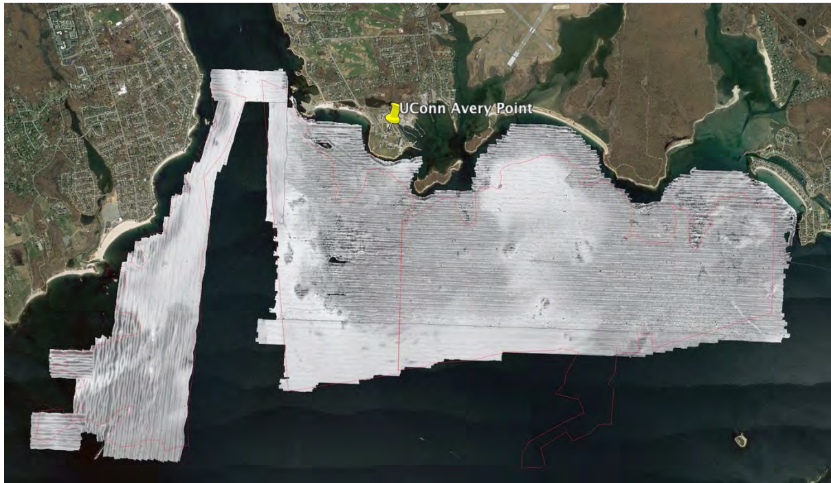
Figure 2.4-2 Mosaic of backscatter data from Survey Blocks 23, 24 and 25 generated by the Geoswath GS4 processing.
