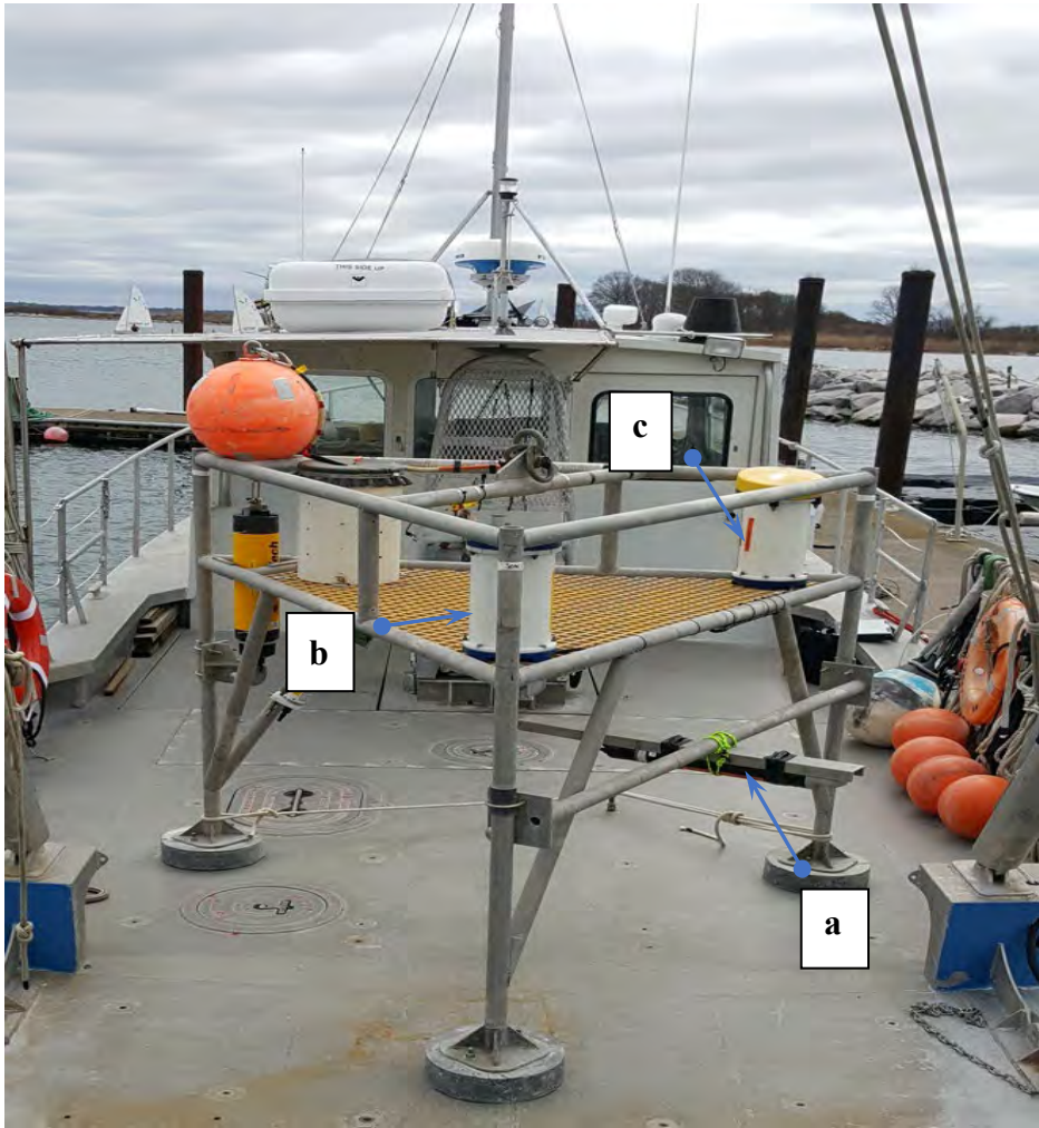
Figure 6.1- 3 Frame deployed at SOW1 – all frames were equipped similarly, with a) Nortek High Resolution downward looking Aquadopp profiler, b) Sea-Bird Instruments Model 37 SMP Conductivity/Temperature/Pressure sensor, and c) RD Instruments acoustic Doppler current profiler with wave array firmware.
