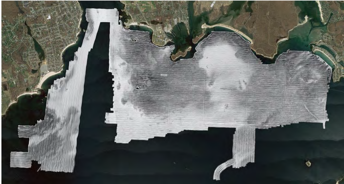
Figure 2.4-5 Mosaic of backscatter data from Survey Blocks 23, 24 and 25 generated by the CARIS processing.
