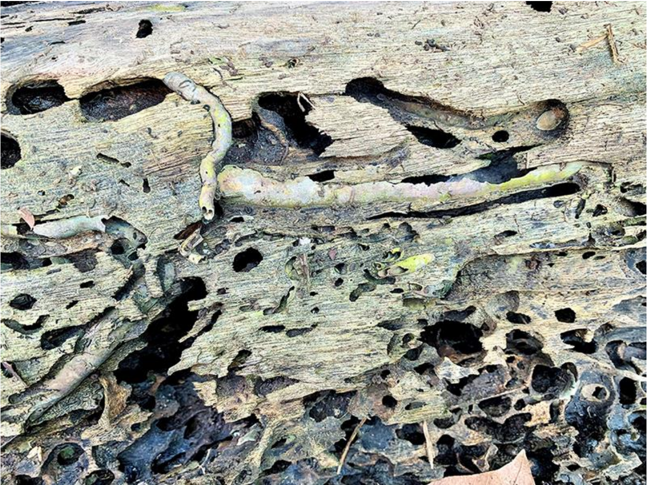
Fig. 1. Decaying tree trunk infested and damaged by shipworms. Calcareous tubes are exposed after the surrounding wood has disintegrated. (Photograph by: Lau Wing Lup).
