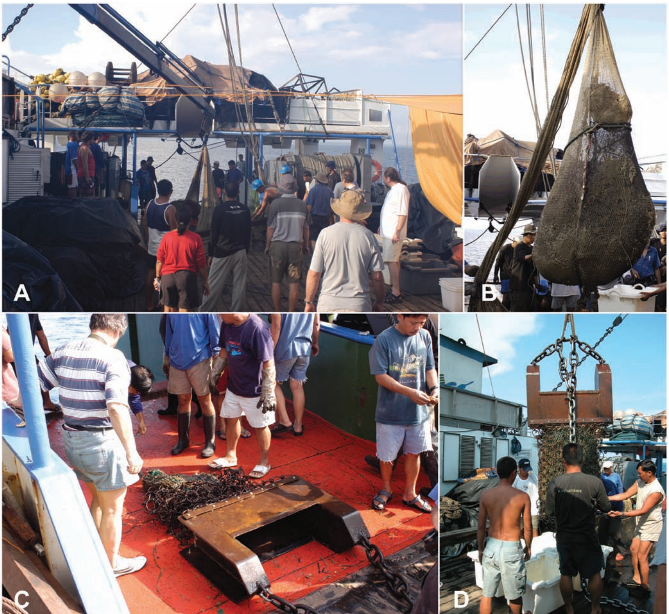
Fig. 4. A, B: Beam trawl on deck after deployment; C, D, Dredge on deck after deployment.
