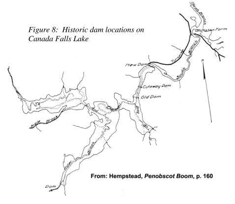
In 1912-13 a new dam with a 26-foot head of water flooded the region behind it, creating the Canada Falls Deadwater. By backing up this water and releasing it at the time of drives, it would exert enough pressure to drive logs to the Seboomook Dam operation. In 1922, the Canada Falls Dam Company built a concrete dam about 100 feet downstream eventually replacing the wooden dam; which was purchased and improved by the Great Northern Paper Company in 1926-27.
