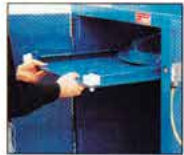
Removable drum crushing platen and a two position key switch to select crush or compact
