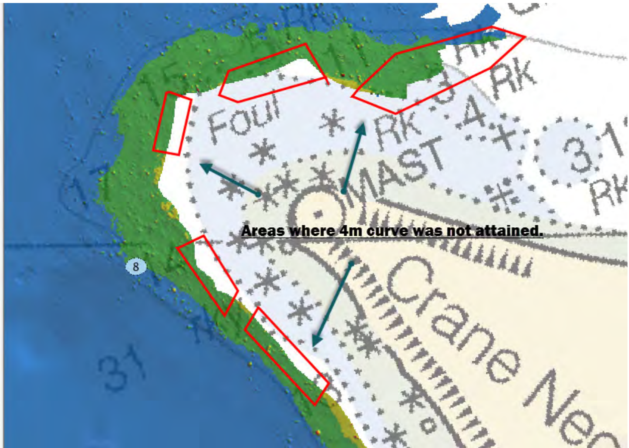
Figure 2: Exception to 4m curve. Green to Yellow denotes 4m curve is obtained
