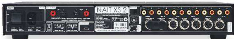
ABOVE: Crowded back panel includes USB upgrade socket, one set of speaker outputs, link plug for power supply upgrade and five RCA/DIN socket line inputs
