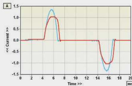
ABOVE: Distorted mains (charging) current waveform (red) versus significantly more linear waveform delivered by the PS Audio P3 Power Plant (blue)
