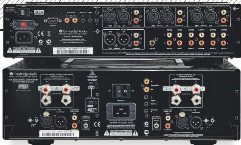
ABOVE: No shortage of analogue inputs here, with lots of single-ended (RCA) and balanced (XLR) options to choose from on the preamp [top]. The power amp can be set to stereo, mono or bridged mono, so you can add more amplifiers down the line
