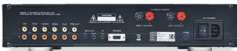
ABOVE: Rear has five line inputs and a preamplifier out, plus IR in/out sockets and RS-232 control port, with a single pair of loudspeaker binding posts
