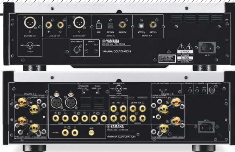
ABOVE: The A-S2100 offers balanced inputs (with switchable polarity and sensitivity), matching balanced outputs on the CD-S2100. Three line, one phono and tape inputs are joined by preamp output RCAs plus massive 4mm speaker cable terminals
