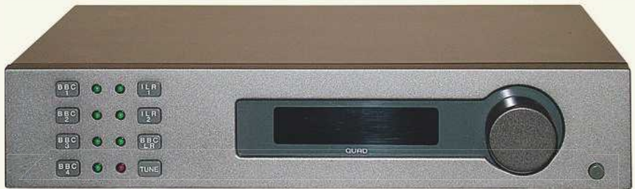
ABOVE: Quad's FM4 was one of the best tuners of the 1980s and offers digital tuning, but a digitally controlled tuner usually features a microprocessor, which can now be difficult to replace
