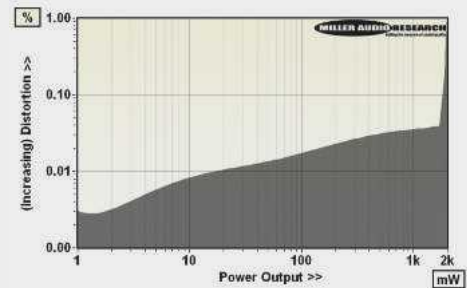
ABOVE: Continuous power output versus distortion (up to 1% THD) into 25ohm 'headphone' load
