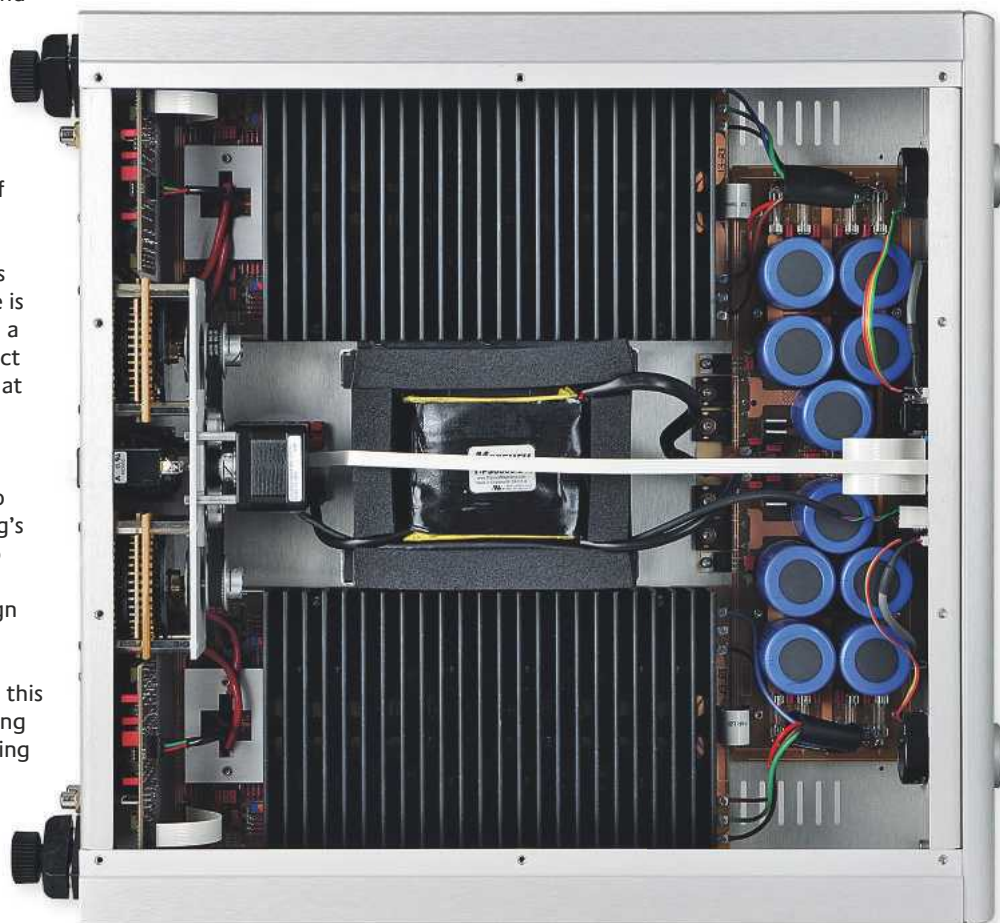
RIGHT: The amplifier modules are embedded under heatsinks but the most remarkable feature is surely the belt-driven stepped attenuator – one for each channel!
