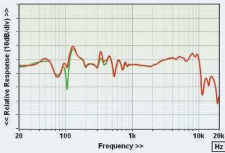
FIGURE 5. Absorbent test, PSB M4U2 (red: right capsule, headband raised; green: right capsule, headband raised, left capsule surrounded by acoustic wadding)
