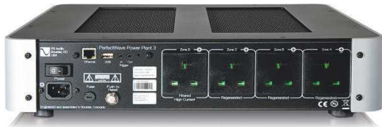
ABOVE: Three of the four output sockets carry regenerated mains, the fourth provides high current capability for larger power amplifiers but is only filtered. An Ethernet socket provides access to extra features via an internal web page
