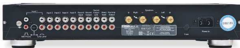
ABOVE: Rear panel sports five line inputs, one switchable between line and MM phono. Rec out, preamp out and a pair of speaker terminals complete the picture
