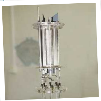
RIGHT: Anode/ Cathode assembly at mid-stage of production. The entire unit has been assembled by hand
