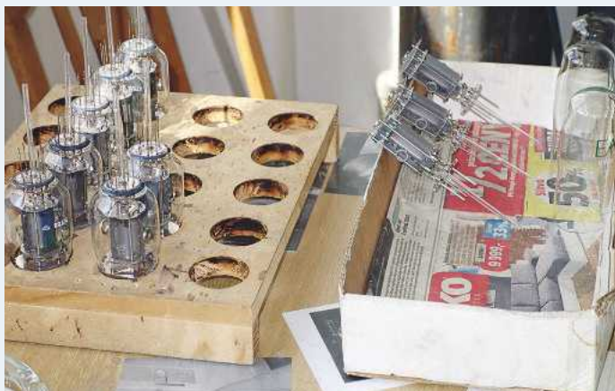
ABOVE LEFT: Finished glass envelopes ready to be fitted with the internal structure
