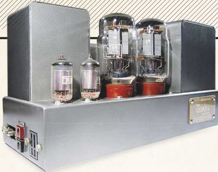
LEFT: Quad II valve power amplifier – rated at 15W on paper, but Richard Oliver wonders whether, on musical peaks, it might sound as loud as a 50W transistor amp
