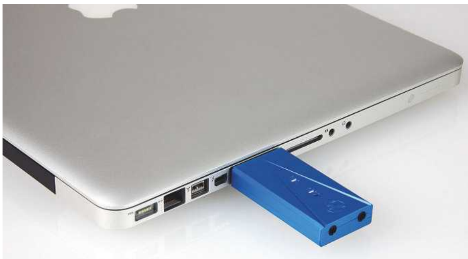
LEFT: Mac and Linux OS need no drivers and plug'n'play via USB; LEDs show sample rate and use of the '3D Awesomifier'. Cans and hi-fi systems are served via dual 3.5mm sockets
