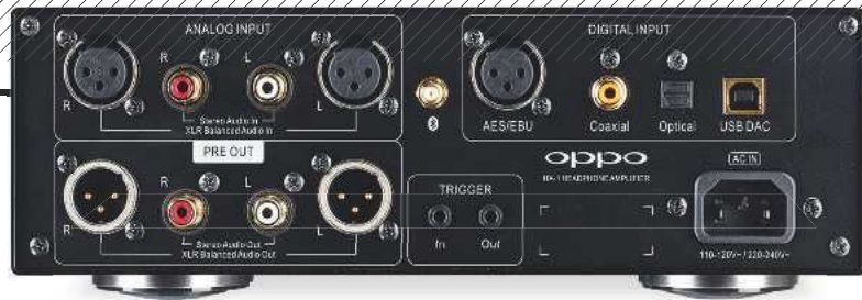
ABOVE: A packed back panel provides balanced and unbalanced analogue inputs and outputs via XLR and phono sockets plus a variety of digital inputs: S/PDIF via phono, balanced AES/EBU via XLR, optical via Toslink, and asynchronous USB
