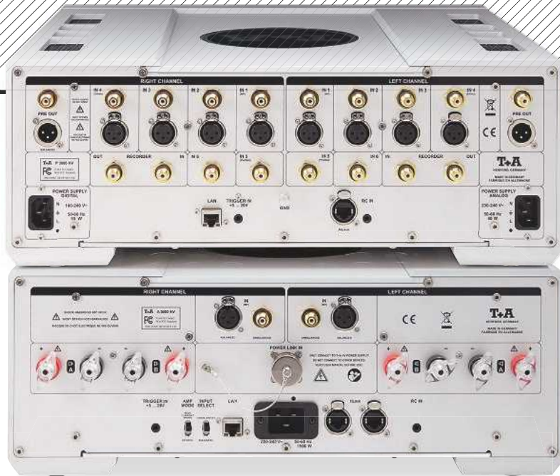
ABOVE: Preamp has six line inputs, four with balanced (XLR) options, a recorder in/out, and balanced and single-ended pre-outs. Power amp has two sets of speaker terminals for bi-wiring or can be switched to 'high current mono' mode
