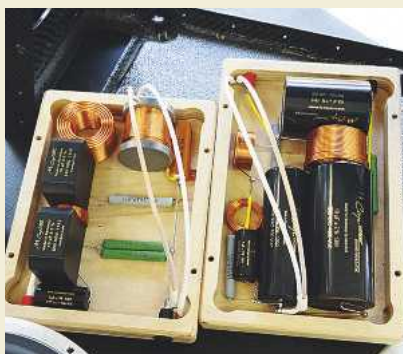
ABOVE: The Mundorf 'Supreme' capacitors used in Sonus faber's new Ex3ma speaker
