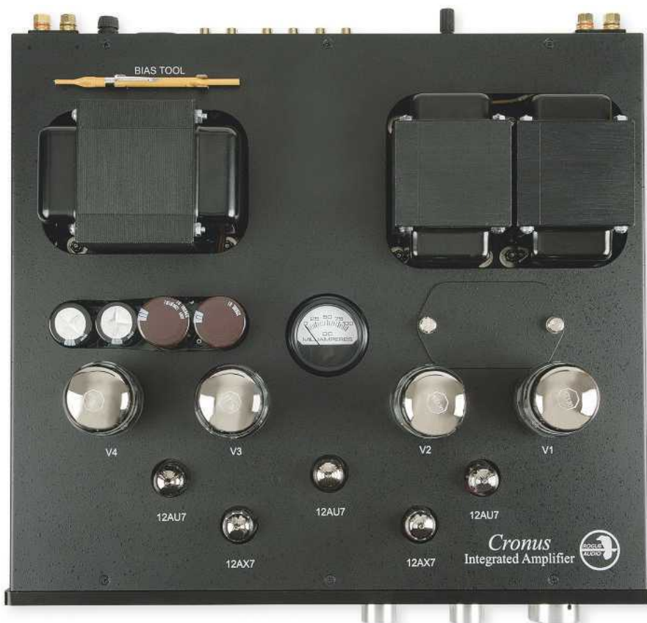
RIGHT: Built-in meter allows setting of DC bias current for the four KT120 power valves. Adjustment pots are situated beneath the removable hatch cover on the right
