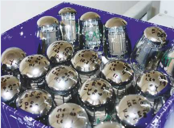
ABOVE: Finished valves awaiting testing and matching; sets are prepared as both pairs and quads for absolutely identical values
