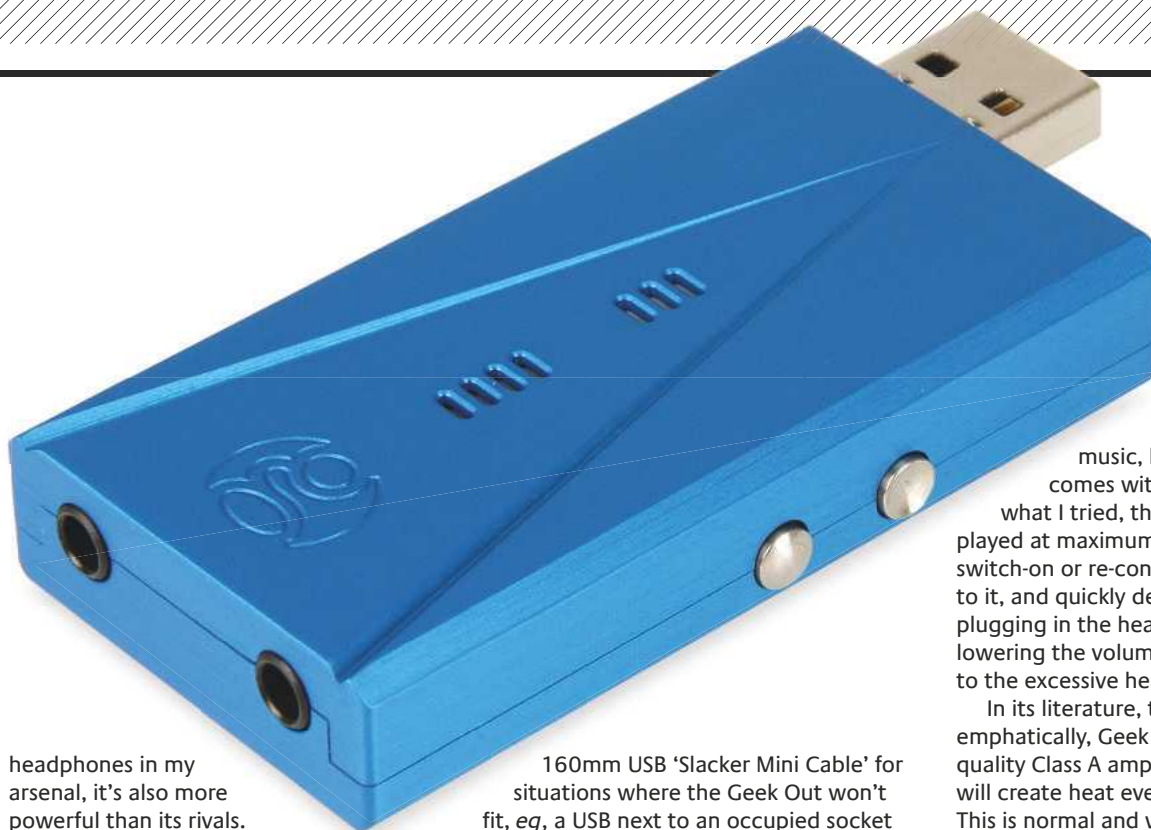
LEFT: Alloy bodies come in different colours according to spec; up/down volume buttons also activate the '3D effect'. The Geek's Class A output causes it to run quite warm
