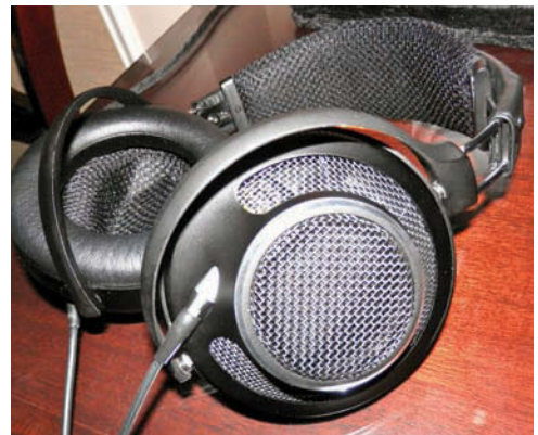
ENIGMAcoustics new Dharma headphones are hybrid electrostats
