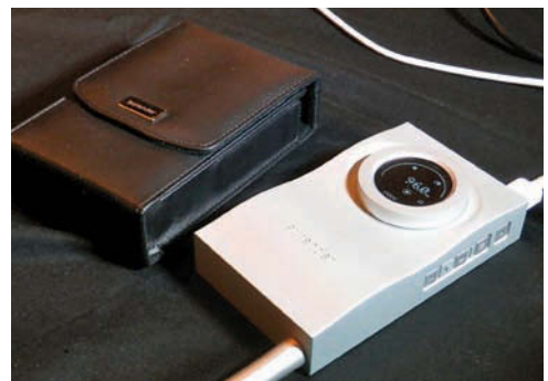
Aurender's first portable device is the new Flow headphone amp and DAC
