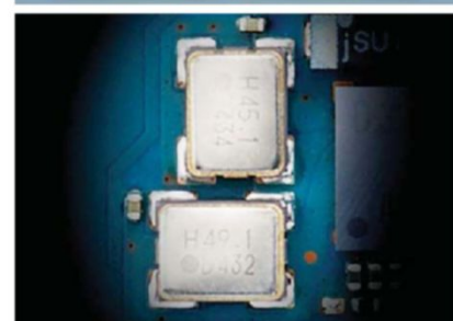
Two dedicated clock oscillations assist synchronized demodulation for top-notch aural performance
