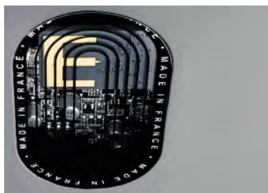
A 'window' on the underside of the sleek casework affords a view of the 110's circuitry
