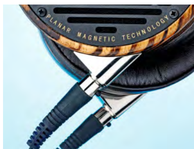
Planar magnetic drive units use a flat diaphragm and an array of magnets to improve resolution
