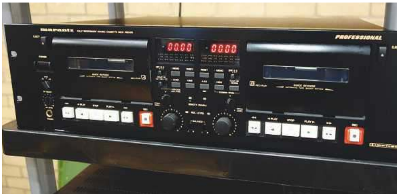
Kicking myself for missing this gem, the Marantz PMD510 Professional Cassette Deck. This robust, studio-grade, rack-mountable unit contained two completely independent, quick-reverse cassette decks with Dolby B and C, CD Sync, remote operation, accurate digital timers and was the choice for those needing to make tape copies within a single chassis.
