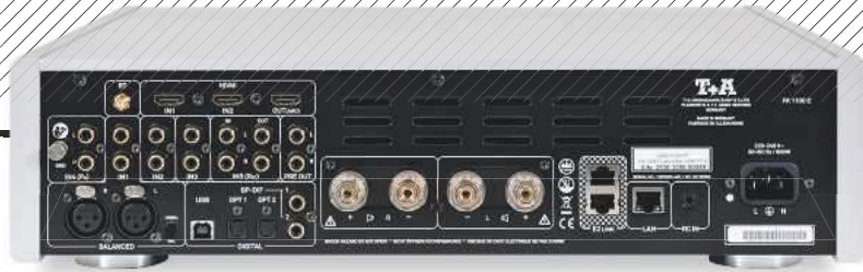
ABOVE: Alongside the tape loop and four line inputs (inc. one balanced XLR and one optional MM/MC phono) are USB-B, two coaxial and two optical digital inputs. HDMI module is also optional. Bluetooth supports aptX but the wired LAN is for control only
