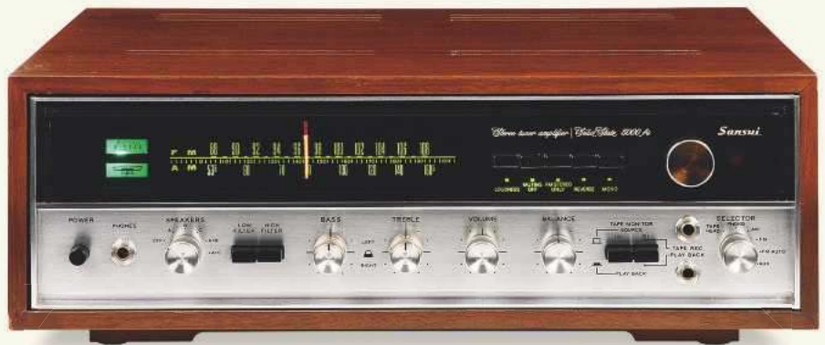
ABOVE: There was no shortage of lights and knobs on the Sansui 5000A from 1969, which employed no fewer than a dozen 6V incandescent bulbs to illuminate the dial and displays
