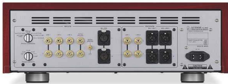
ABOVE: Four line ins (inc. one balanced on XLRs) are joined by one phono in (on RCAs) with rotary MM/MC gain and loading options. Four line outputs are offered on single-ended RCAs and balanced XLRs. The CL-1000 has no remote control
