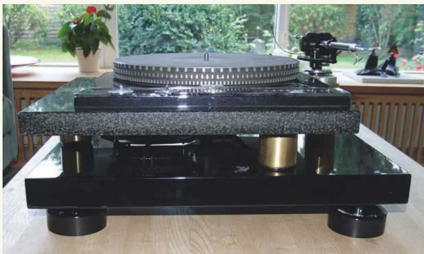
ABOVE: Reader Alan Ericsson's refurbished and modified Garrard 401 turntable which sports a granite stone upper plinth supported on a lower plinth of 40mm-thick MDF
