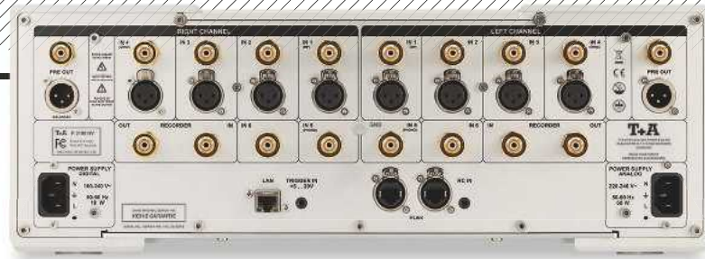
ABOVE: Separate IEC mains inlets for 'analogue' and 'digital' (switching/display) PSUs are fitted alongside six line inputs – four on balanced XLRs, one with a MM/MC phono option – a tape in/out, and balanced and single-ended preamp outputs
