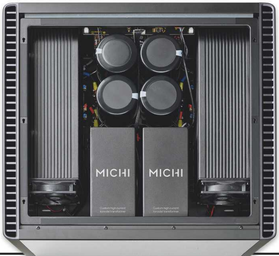
RIGHT: The M8 includes a pair of epoxy resin-filled transformers and four UK-sourced 47,000µF PSU reservoir caps. The Class A/B output stage has 16 pairs of high-current power transistors on two fan-assisted heat pipes
