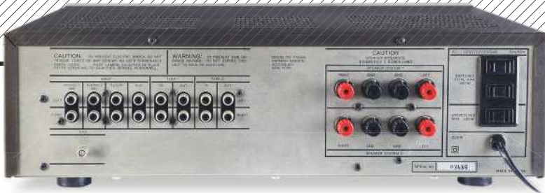
ABOVE: Rear panel sports sturdy binding posts for the speaker connections while the inputs are all standard RCAs, well spaced to suit modern cables. Note the US-type mains outlets above the captured lead – most manufacturers chose to blank them off
