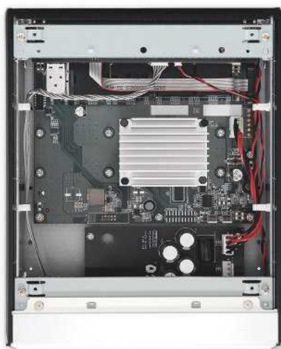
ABOVE: The 12V/4A external supply is routed through to additional regulation [bottom] while the mainboard processor is screened and cooled under a heatsink
