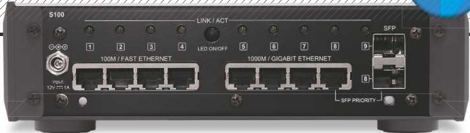
ABOVE: Ten ports populate the rear of the S100 – four each of 100Mb and 1000Mb (1Gb) and two optical fibre SFP (small form-factor pluggable). The 100Mb ports are recommended for 'straight' audio, the 1Gb links for PC/Roon Core applications
