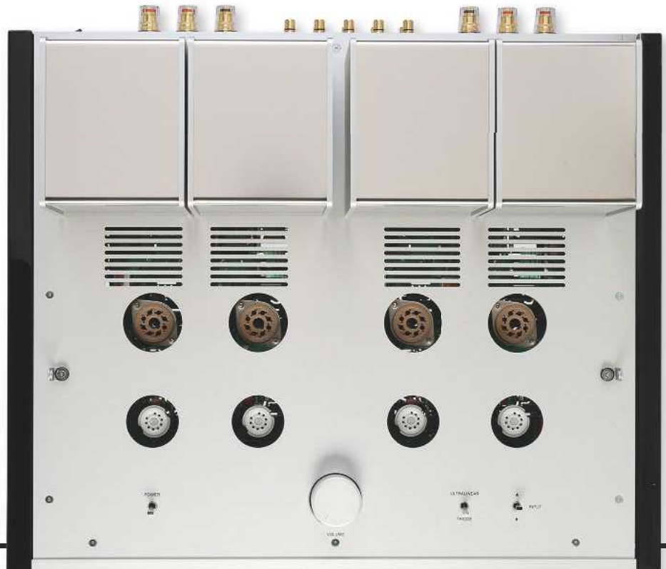
RIGHT: Overhead picture shows the seats for the pairs of 12AX7 and 12AT7 triodes and larger 'Kinkless Tetrode' KT88 pentodes. The latter may be configured for triode or ultralinear output modes, on-the-fly, via a toggle [lower right]
