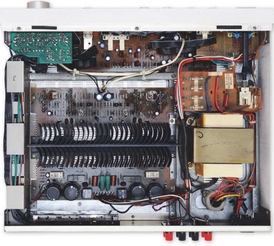
LEFT: Unusually for a powerful amplifier of this era the PM650 has an internal heatsink. Note the large mains transformer and dual power supplies necessary for high current operation
