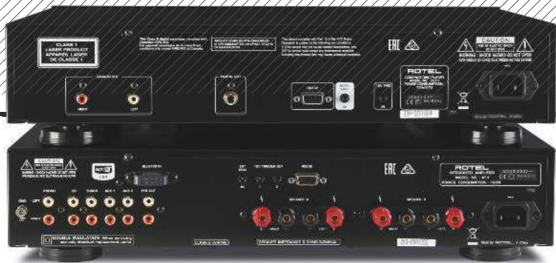
ABOVE: Bluetooth, MM and four line ins join pre outs and two sets of (switched) 4mm speaker cable posts on the amp [top]. CD player [bottom] has no digital inputs – just analogue outs on RCAs and S/PDIF out on coax. Note trigger and RS232 control ports
