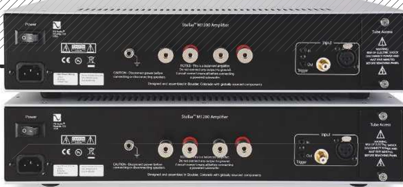
ABOVE: The M1200 offers balanced (XLR)/single-ended (RCA) ins alongside parallel sets of 4mm speaker outlets (these are ‘floating’ so must never be connected to gnd., such as an active sub). Note removable panel for access to the triode tube [far right]
