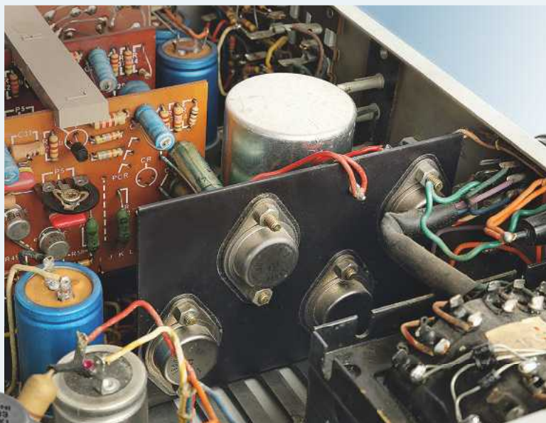
RIGHT: RCA 2N3055 output transistors [centre of image] inside Leak's Stereo 30 Plus amplifier [HFN Sep '20]
