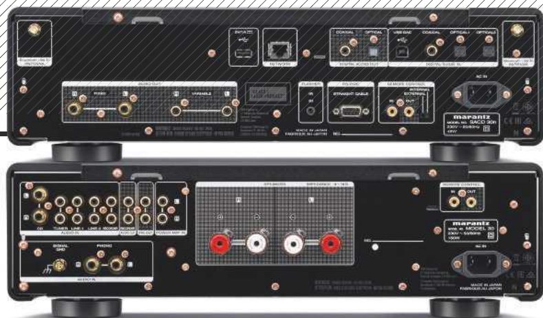
ABOVE: SACD/network player/DAC [top] has wired Ethernet, BT, coax/two optical and USB-B/USB-A digital inputs plus optical/coax digital outs and fixed/variable analogue outs on RCAs. Amp [below] has MM/MC phono plus four line ins, a tape loop, pre out/power amp in and 4mm speaker binding posts
