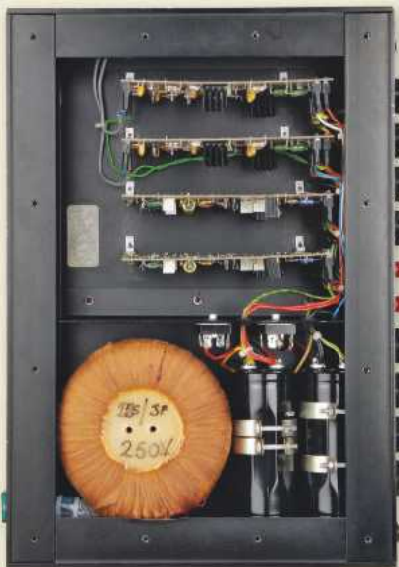
ABOVE: Original Naim NAP250 amp from 1975 used BDY58 transistors from Solitron
