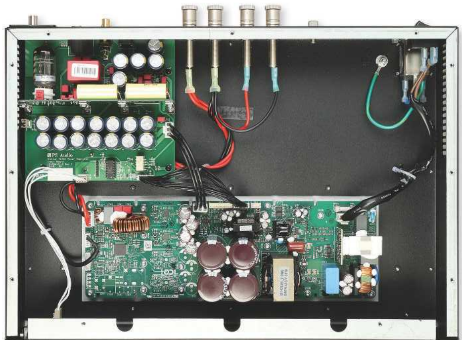
RIGHT: The M1200 combines a 12AU7 triode tube-based line input [top left], fed from a linear PSU, with an ICEpower ICEEdge 1200AS1 mono Class D amplifier module [bottom], incorporating its own switchmode PSU
