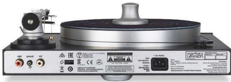
ABOVE: Tonearm bias weight is readily adjustable as is tonearm height (VTA). The AC-DC PSU is built into the chassis, as is the electronic speed selection, but there is no fine speed control. Tonearm wiring exits in RCA's with a ground post in between
