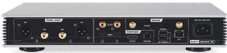
ABOVE: Digital ins include wired/wireless Ethernet and I 2 S on an HDMI socket (up to 768kHz PCM, DSD256 as DoP and DSD1024 natively), USB-B (also 768kHz PCM and DSD256 as DoP), 2x optical/coax S/PDIF and external files via MicroSD and USB-A. Analogue outs (fixed or variable) are offered on RCAs and balanced XLRs
