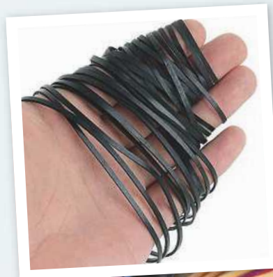
BELOW: A sticky belt inside an Aiwa AD-R450 cassette deck. Replacement belts are readily available online
