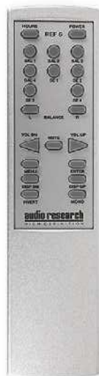
LEFT: Partnering remote caters for input selection, mono, mute, volume, balance, phase invert, and access to limited menu functions
