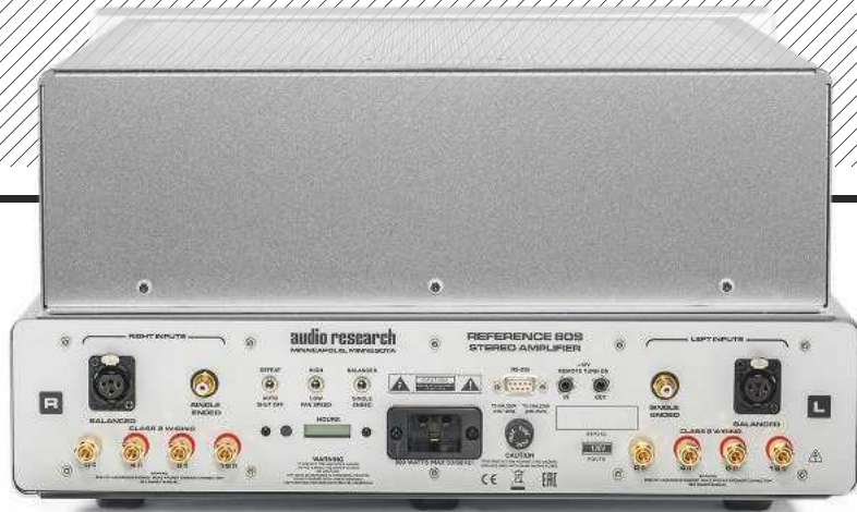
ABOVE: Small toggles switch between single-ended (RCA) and balanced (XLR) inputs, fan speed and auto-shut off (signal sensing). Tube hours are indicated beside a bladed IEC mains inlet, while 4mm speaker binding posts offer 16ohm, 8ohm and 4ohm taps
