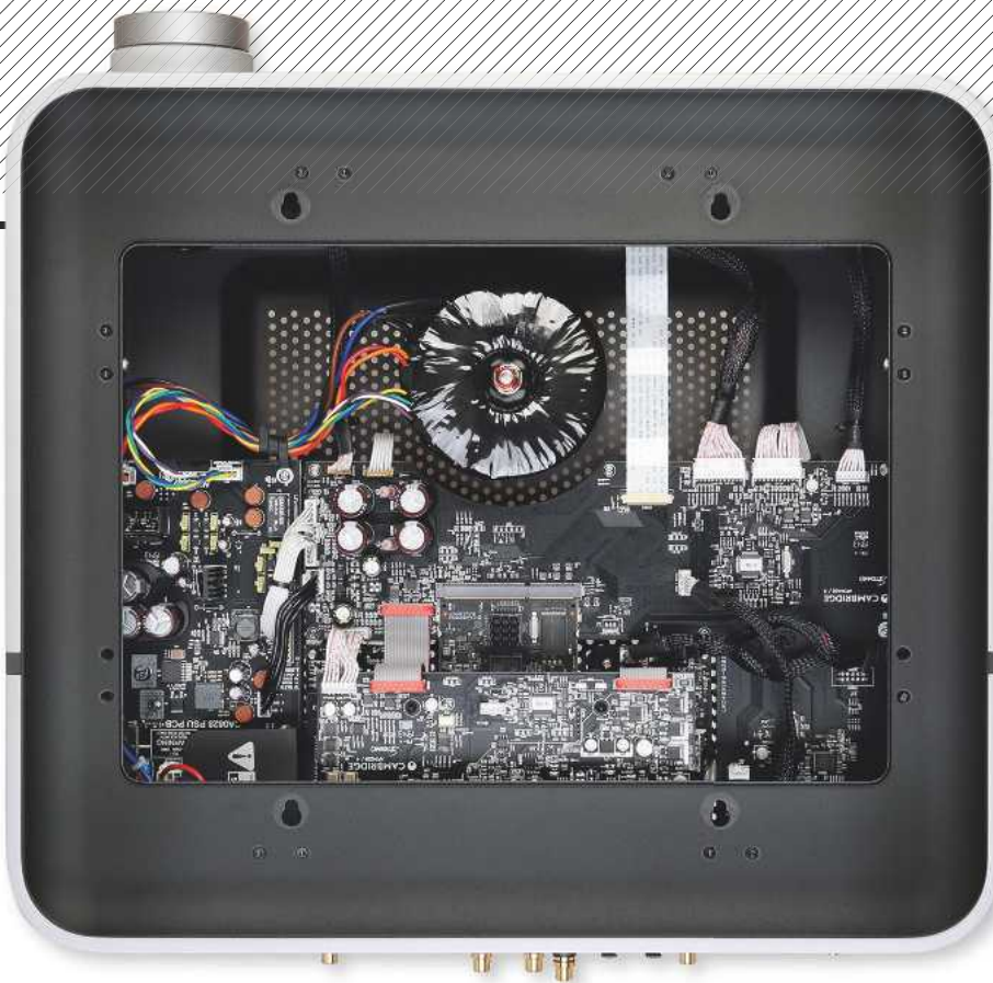
ABOVE & BELOW: The Edge NQ's toroidal transformer [top] feeds multiple PSUs. The StreamMagic 'Black Marlin' streaming platform [centre] is the NQ's beating heart – and controlled via its own app [see bottom of page] – while an ES9018 DAC forms the core of its balanced output stage [bottom]
