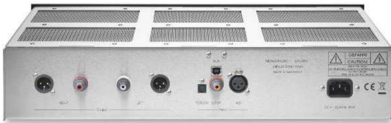
ABOVE: Simplicity itself as the DAC1 offers a single USB-B port (also I 2 S in the future), one balanced AES/EBU alongside S/PDIF on optical and coaxial inputs. Fixed-level analogue outputs are offered on XLRs (balanced) and RCAs (single-ended)
