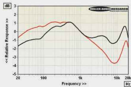
ABOVE: Freq. resps (-8dB re. 5cm/sec) lateral (L+R, black) vs. vertical (L-R, red). No RIAA correction >2kHz
