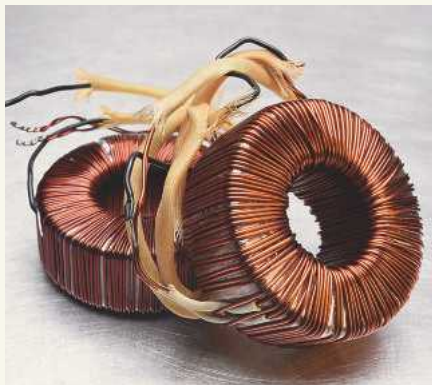
ABOVE: Typical toroidal mains transformers as used in many audio power supplies today
