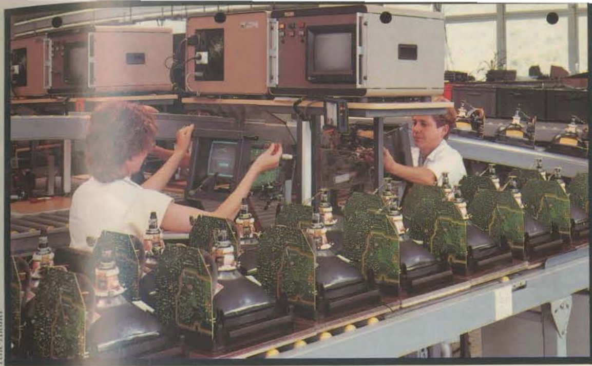
Every Minitel is part computer and part video, and is test run. Here the video portion is adjusted to ensure a sharp picture.
