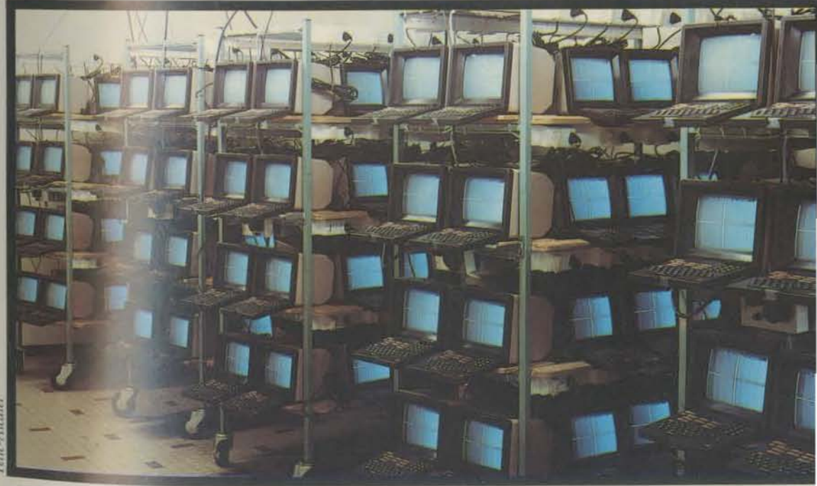
After individual testing, Minitels are stacked on mobile racks and subjected to a temperature-control environment.
