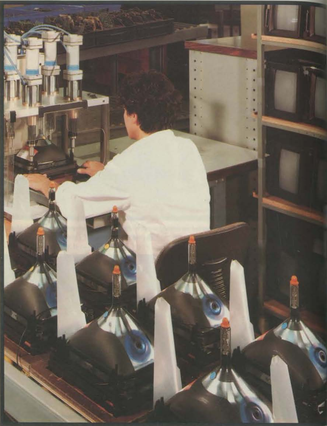
A semi-automatic assembly line. Without housing, Minitels look like over-sized insects ready to take flight.
