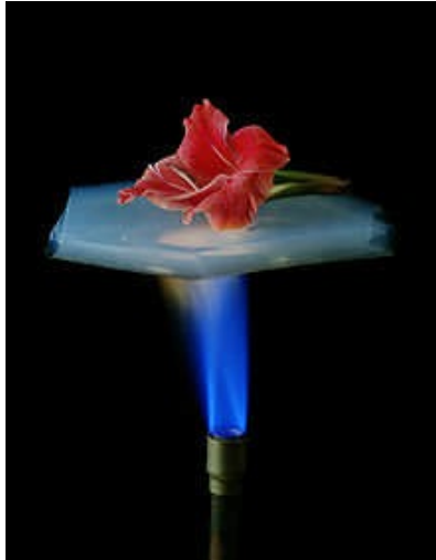
Flower atop a monolith of aerogel with a flame from a torch beneath
