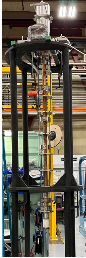
Figure 17. High efficiency 1.3 GHz klystron assembly without the surrounding solenoid.
