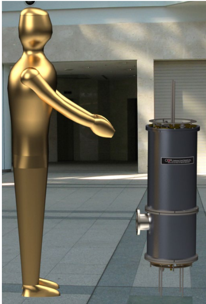
Figure 14. Rendering of a 200 kW, 350 MHz multiple beam triode RF source model.
