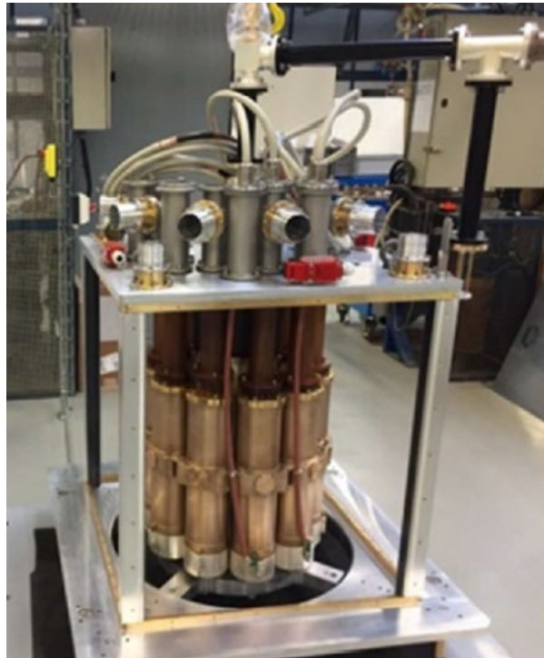
Figure 18. Input coupler for CPI MBIOT for the European Spallation Source.
