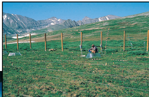
ABOVE: In the snowpack enhancement study at Niwot Ridge LTER site, the depth and duration of the snowpack is altered by the fence. This long-term project (International Tundra Experiment, or ITEX) is conducted at several sites across the LTER Network (photo: T. Seastedt).
