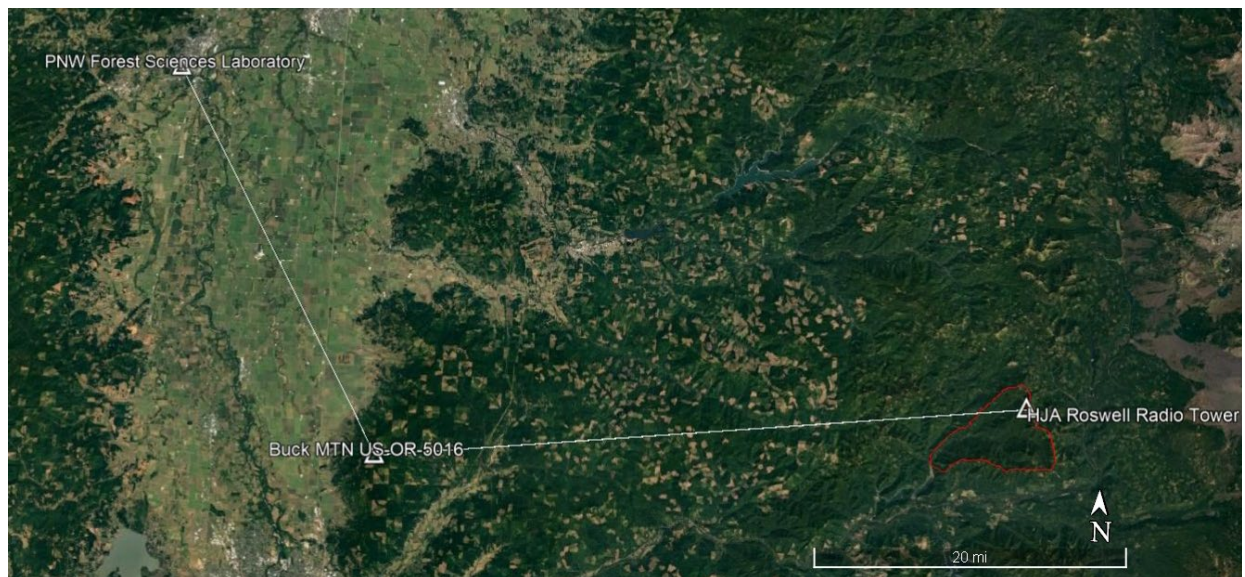
Figure 1-Facilities. Wireless communication infrastructure (A) within the H.J. Andrews Experimental Forest – HJA and (B) linking HJA to the OSU campus and USFS PNW Research Station in Corvallis, Oregon.
