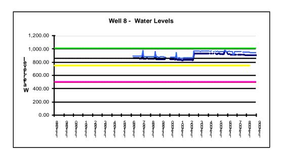
Green - Initial Water Level; Yellow - Action Level; Red - Lowest Allowable Level; Pink - Trigger for Designation Proceedings; Dotted - Pump Level, Thick Blue - Low Water Level; Thin Blue - High Water Level
