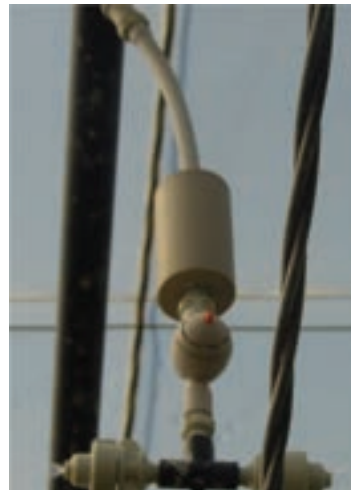
Photo 14. Low pressure nebulisation nozzle
