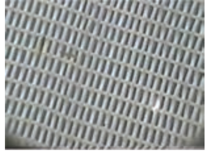
Photo 10. Mesh 28 x 14 threads/cm 2
