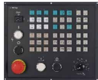
Control Panel for Mill
