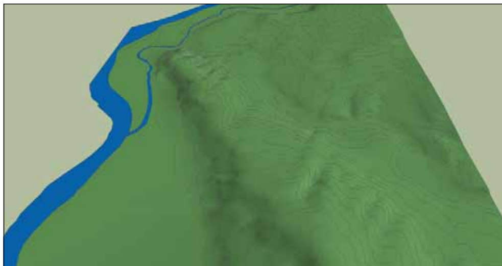
8 A three-dimensional terrain model of the surrounding area of Zrínyi-Újvár from a bird's eye view from the south, constructed from the 1: 10,000 military contour-map
