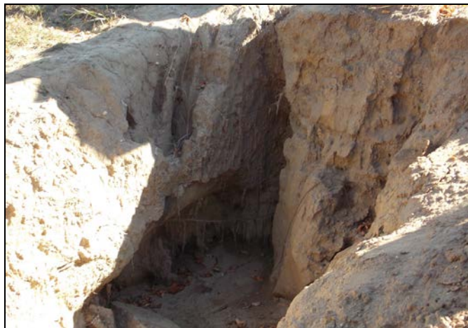
Figure 6: Association between suffusion and rill erosion with steps of 40-50 cm forming.
