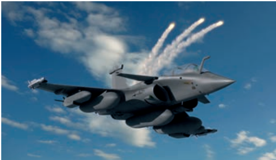
Forward-firing flares are intended to outfox the ECCM capabilities of IR-guided missiles, which may be designed to discount flares travelling in an aircraft's wake. (Photo: Etienne Lacroix)
