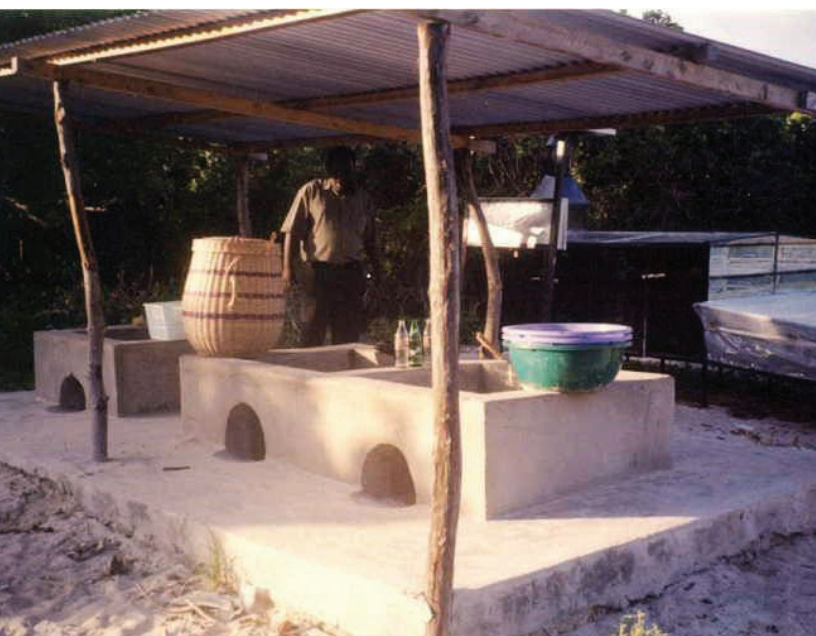
Improved blocked smoking oven in Gazi
