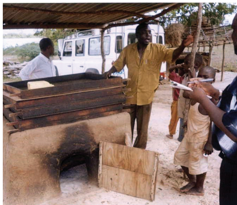
Improved clay walled single door oven in Moa
