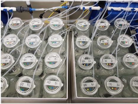
Experimental tanks aerated with an air/CO 2 mix to simulate end-of-century ocean acidification conditions.
