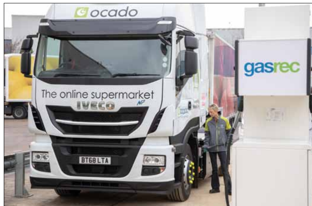
◀ Biomethane has a role to play in the low-carbon transition. This CNG refuelling station in Hatfield, UK supplies blended biomethane to delivery trucks.
