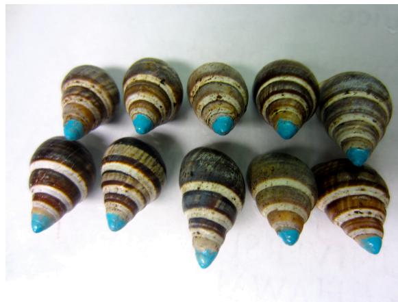
Figure 7. Xylene paint environmental test. In order to experimentally determine durability of paint pen on Achatinella mustelina shells we painted dotted 10 shells on June 27, 2012, then placed shells in a screen cage in an environmental chamber. This photo was taken after 4 months of exposure to chamber conditions including 3 minutes of sprinkler spray every 8 hours. Paint is still bright and intact.
