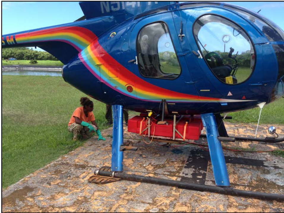
Staff inspecting the spray rig prior to beginning aerial operations
