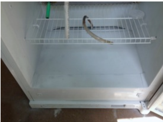
Figure 1. Chamber refurbishing and maintenance. Photo labeled A shows rust penetrating the frame of the chamber, where door hinge failed. Photos B and C depict a typical rusted chamber floor and door with light fixture. We moved the chamber outdoors, treated for rust, scraped with
