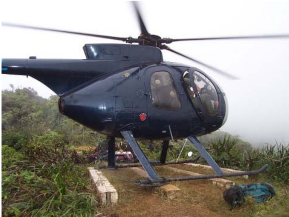
Typical constructed helicopter LZ
