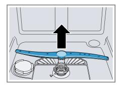
3.Check the outlet nozzles of the spray arms for blockages under running water and remove any foreign bodies.
