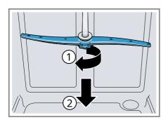
2.Pull the lower spray arm upwards.
