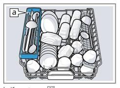
knife rest a<sup>1</sup> To create space for larger dishes, you can adjust the height of the upper dish rack.
