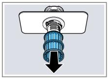
4.Press the locking lugs together and ① remove the coarse sieve upwards. ②
