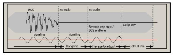
The breakdown of the TM8100 encoded transmit audio and subaudible signalling can be seen above where values are set in the TM8100 PC Application as defined below:
