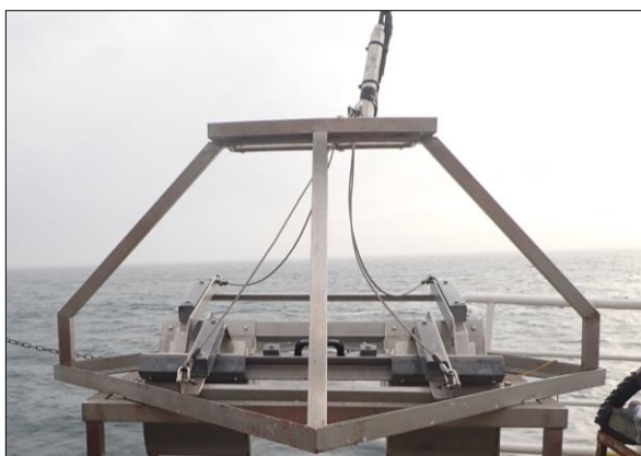
Figure 9 Dual Van Veen grab sampler.
