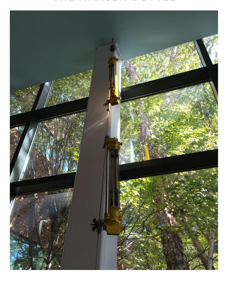
The Nansen Bottle was developed in 1894 by oceanographer Fridtjof Nansen and was used in oceanography until about 1981. It was mounted on a wire lowered from a ship and used to sample water and measure temperature at depth. The Nansen bottle is the precursor to Niskin bottles currently used in oceanography.
