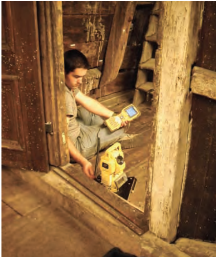
Joshua Marano operates a total station during the 2010 Vasa recording project.
