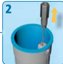
Lift float with cable to simulate fill
