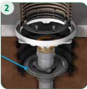
2 Remove Lower Bolts and Ring and Remove Bellows
