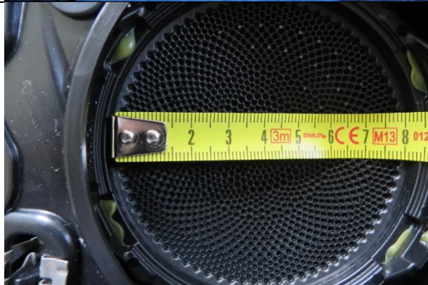
Perforated grill in doorpanel is 80 mm
