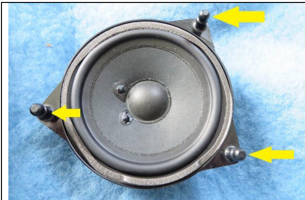
Unclick the speaker from the doorpanel (3 rubberhosted clickpoint – see yellow arrows)
