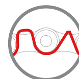
ASYMMETRIC TOOTH DESIGN PROVIDES SMOOTHER CHAIN ENGAGEMENT
