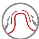
CHAMFER ON THE TEETH HELPS SHED MUD
