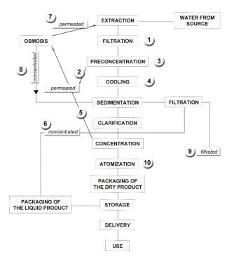
**Figure 2.** Operating diagram of extraction and fractionation plant from Reference [87], consisting of (1) filtered tannin broths; (2) permeate from nanofiltration Step 1; (3) concentrate from nanofiltration Step 1; (4) concentrate from nanofiltration Step 2; (5) permeate from nanofiltration Step 2; (6) concentrate from nanofiltration Step 3; (7) osmosis permeate; (8) osmosis concentrate; (9) settled fraction from clarification step; (10) spray-dried obtained from fraction 6.
